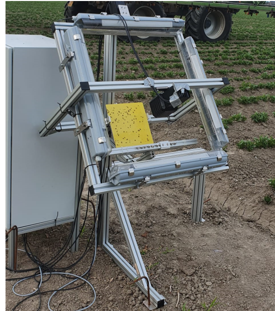
Fig. 1. The new approach captures flying insects using a camera directed at a yellow sticky plate. This setup includes LED bars, a trigger, and a line-scan camera recording at 1936x2 resolution. When an insect disrupts the trigger's light, the main camera captures a focused image illuminated by flashing LEDs for 133 \mu s, saving it at 4512x4512 pixels resolution. The camera was strategically placed on several Frisian farms to capture the necessary data.
